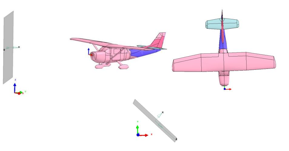
RCS simulations of the Cessna showed an advantage of Co-Polarized signals, especially in areas where specular reflections on the airframe happens.
